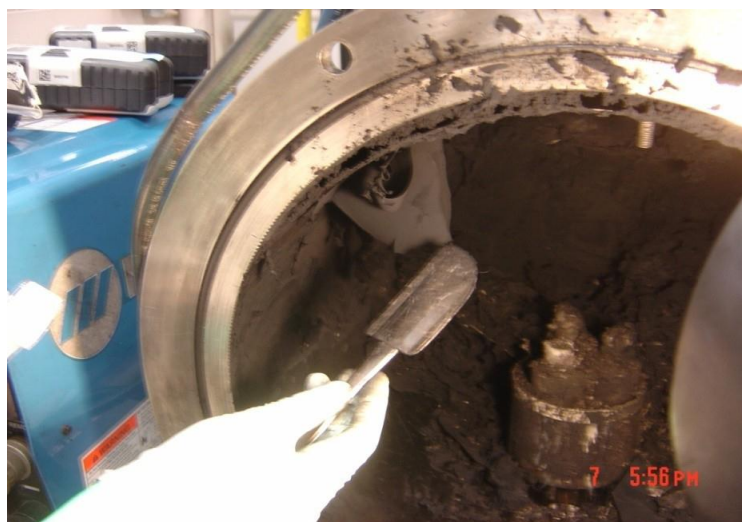
Figure 4. The manual transfer of carbon nanotubes from a production vessel (courtesy of PA Schulte, National Institute for Occupational Safety and Health [NIOSH]).
