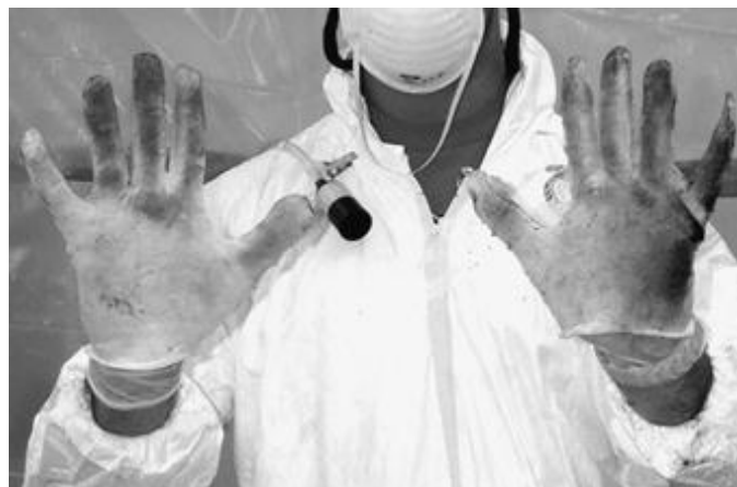
Figure 6. Protective gloves contaminated with very fine carbon nanotube dust (courtesy of A Maynard, NIOSH, Baron et al., 2003)
