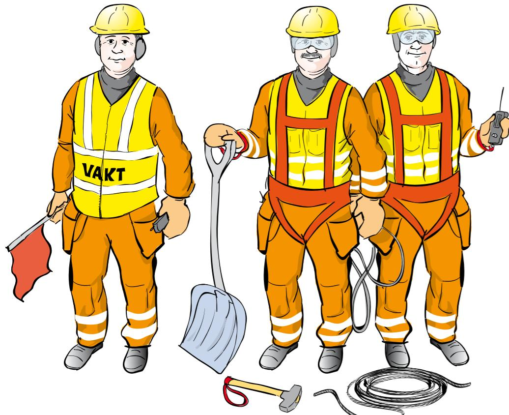
**There should normally be two persons on the roof when shovelling snow. One person is to move the anchorage points for the line and keep it taut while the other is to carry out the actual shovelling.**
