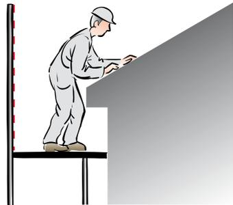
If fixed protection cannot be installed, personal safety equipment with a harness shall be used. A waist belt can cause serious injury and shall not be used. Secure the safety line to a permanent structure on the roof. Check that the attachments are reliable. If a safety line cannot be attached anywhere on the roof, it may be wound around a permanent structure and held taut by another person.
