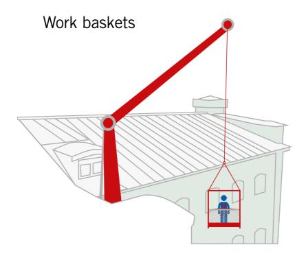
There are different types of work baskets. The basket is often fixed or temporarily mounted on a vehicle. For some cranes and forklift trucks one can use a temporary work basket. The basket should be used and designed according to current regulations. This entails also that the user needs to have special competence.
