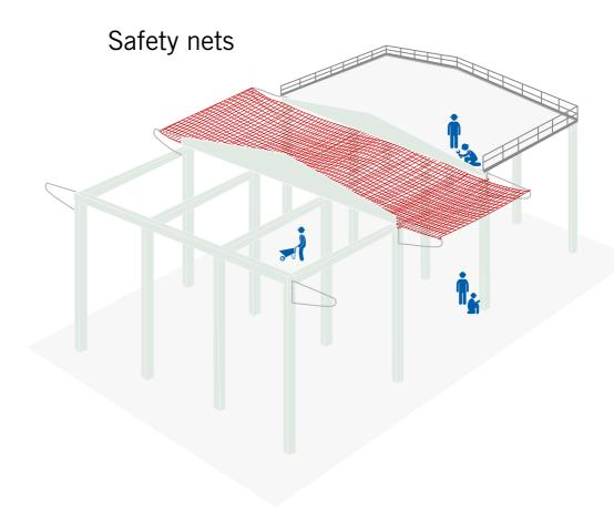
Safety nets should be designed so that they can safely catch a person that falls and at the same time prevent the person hitting something underneath the net. The safety net should be assembled and checked by persons with special knowledge about safety nets.
