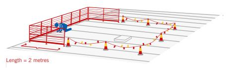
If the roof is flat with a pitch of 6 degrees at the most, you can choose a simpler protection against the risk of falling from height. The following must be fulfilled:
