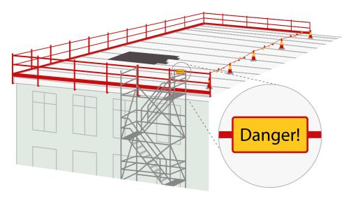
When there is a risk of falling through a roof, it must be investigated before the work can start. Areas where there is a risk of falling through a roof must be closed off with clear and durable barriers. Often, clear barriers on access routes are also required.
