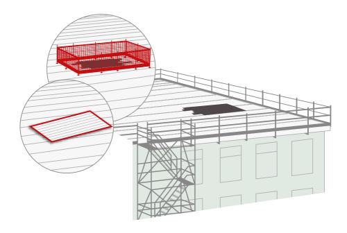
Openings and holes with a risk of falls from height must be protected by a fall protection guardrail, or covered. It is important that the guardrail is designed according to the description for guardrails. The guardrail must be around the entire opening. If one chooses to cover the hole with a slab or equivalent, is must be durable, stable and be clearly marked. Where there are lifts or other heavy vehicles that could drive in the vicinity, the covering or guardrail must be adapted accordingly.
