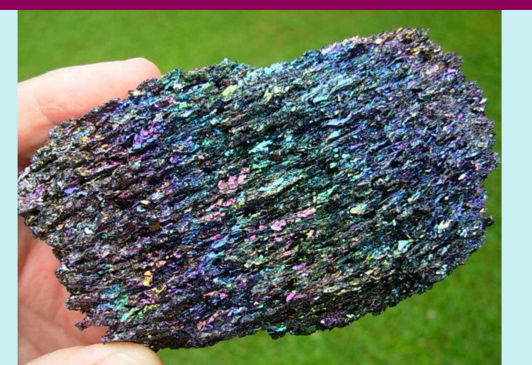
Figure 1. Piece of crude SiC (left) and close-up (right)
