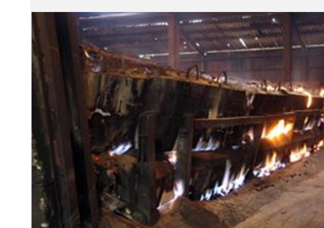
The burning process lasts 40-170 h whilst the core reaches ≈2500°C. Above 1700°C, silicon in the quartz and carbon in the coke combine to form SiC and CO:
