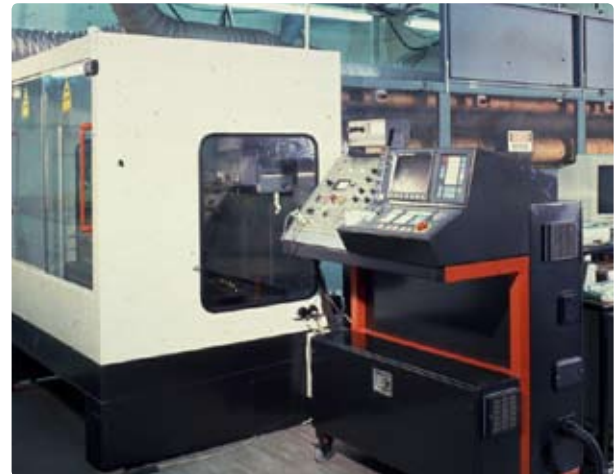
Vision panels in guarded area
